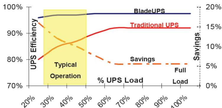
**Figure 5.** Efficiency savings with the Eaton BladeUPS.
