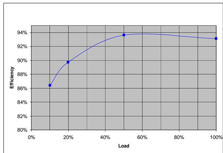
**Figure 3. Vendor A: 1000W PSU operating at 240V.**
