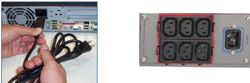
**Figure 4.** Remove the input cable from your IT equipment and simply plug it into the input IEC receptacle of the UPS (blue circle). Use the various jumper cables provided with the UPS to connect the IEC outlets of the UPS (red) with the various IT devices you want to protect.
