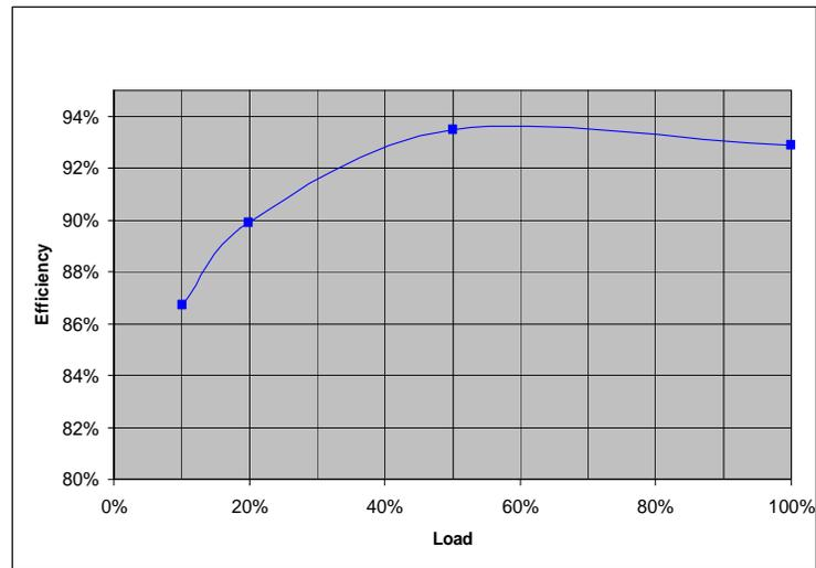
**Figure 2. Vendor A: 1000W PSU operating at 230V.**
