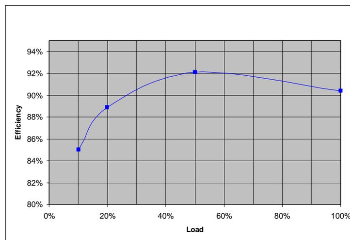
Figure 1. Vendor A: 1000W PSU operating at 115V.
