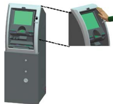
Figure 4: ATM for convenience stores with small palm vein pattern authentication sensor unit (CG design image).
